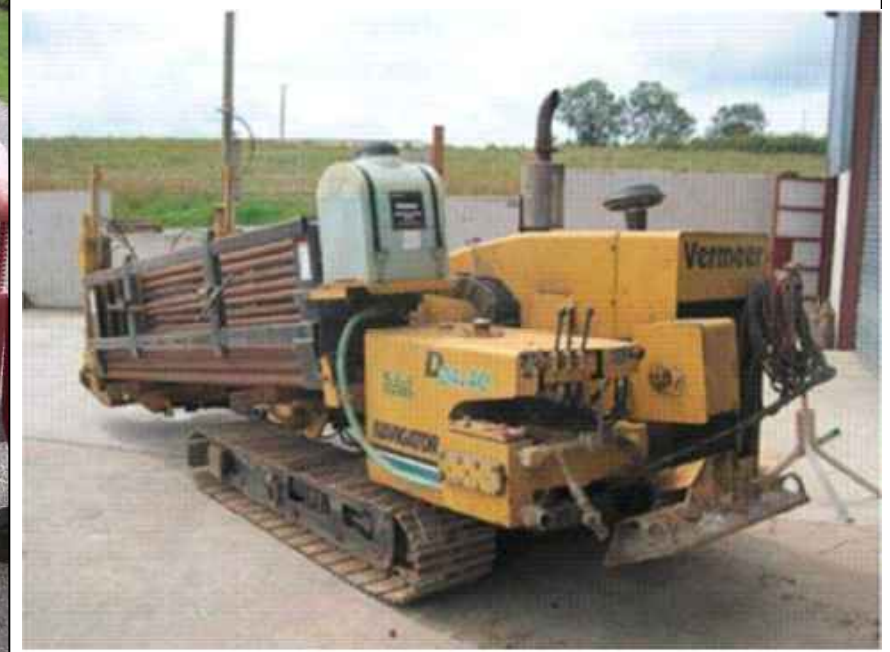
Typical Directional Drilling Rig
